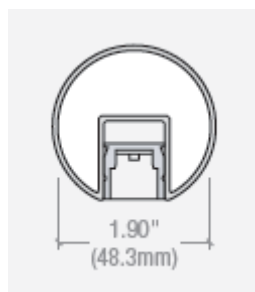
Figure 1.5: Lobby Handrail Detail
